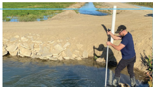
Matt Dermody takes a reading with a staff gauge at the weir where a grower is taking water. The difference between measurements taken above and below the weir reveals how much water is used.
