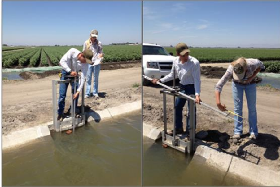
Figure 16. Custom-made tool used to measure actual gate opening
