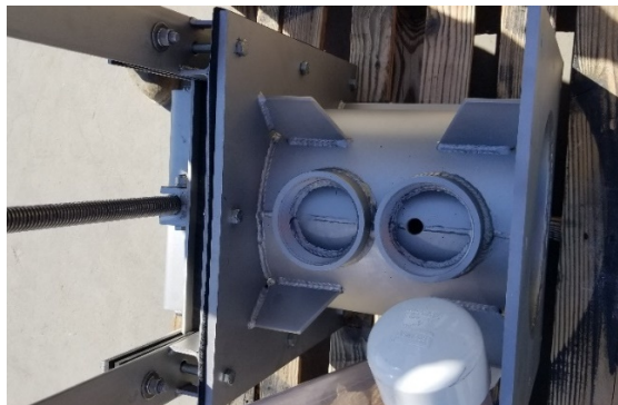
Figure 22. Top view of prefabricated canal metergate (Fresno ID, 2019)
