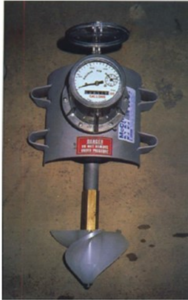
Above, propeller flow meter, the most common flow meter used for irrigation pumping plants. Below, flow meter installed in test section used for this study.
