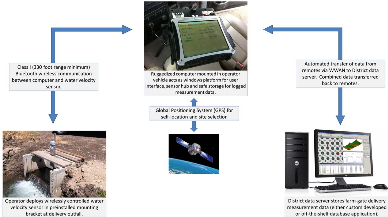
Figure 2. RemoteTracker Principles of Operation Overview
