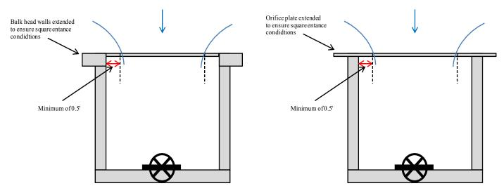
Figure 5. Installation of orifice
