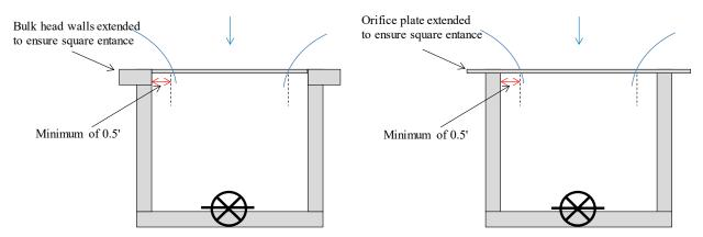
Figure 27. Guidelines for orifice entrance extensions
