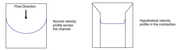
Figure 37. Parabolic velocity distribution without a contraction (left) and theoretical velocity distribution with contraction installed (right)
