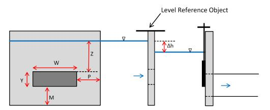
Figure 26. Dimensions for fully contracted submerged rectangular orifice
