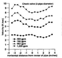
Fig. 2. Water velocity profiles under a check valve.
