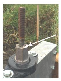
Figure 17. The "zero" opening mark ground into the threaded rod
