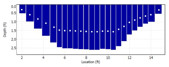
Figure A-7. SonTek ADV Cross Section for Canal Verification Measurement
