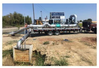
Figure 13. USBR/ITRC Irrigation Turnout Calibration Unit
