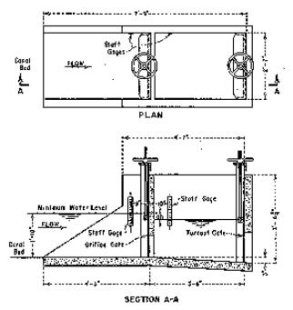
Figure 29. Schematic of a USBR CHO (from USBR, 2001)
