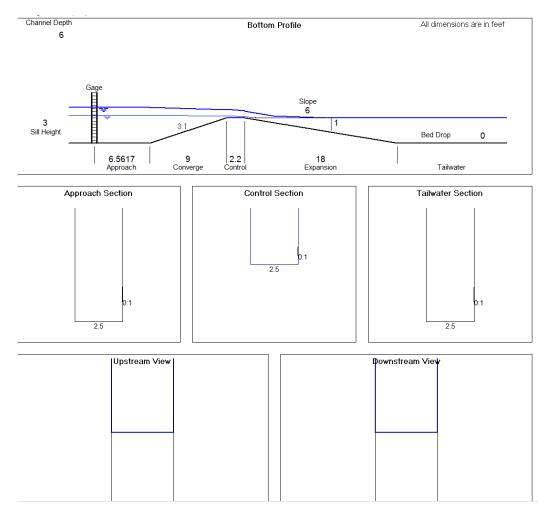
Figure 45. Example output from WinFlume<sup>™</sup> for a typical Replogle flume. This has rectangular side walls.
