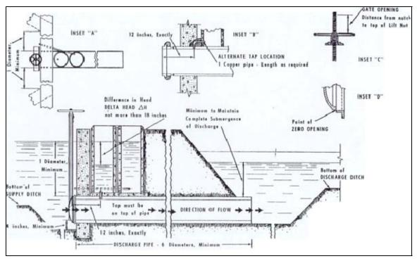
Figure 8. Photo courtesy of an old Armco flow measurement catalog. This depicts a common "metergate" with very specific dimensions that must be met if the rating tables are to be used.
