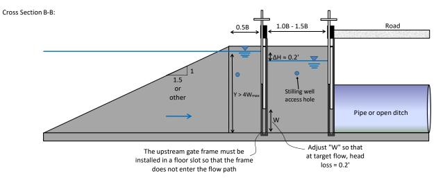
Figure 31. Side view of CHO on lined canal bank. Not to scale.
