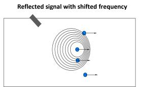
Figure 34. Doppler shift caused by moving particles in the water
