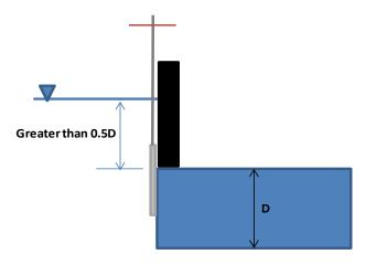
Figure 15. Minimum upstream submergence above the top of the gate
