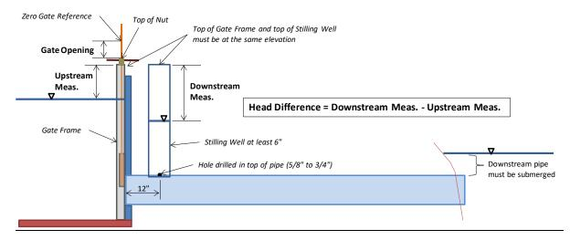
Figure 14. Proper metergate dimensions – but lacking precast design.
