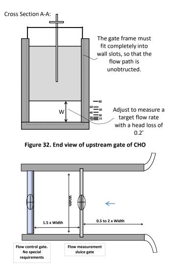
Figure 33. Plan view of CHO constructed in earthen canal. Not to scale. Rounded entrances are recommended.
