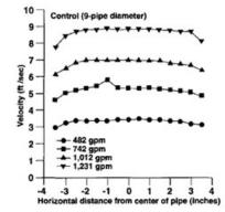
Fig. 1. Water velocity profiles under control conditions.
