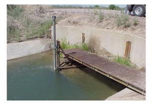
Figure 8. Open propeller meter installed at the discharge end of a large full turnout pipe. Water flows from right to left
