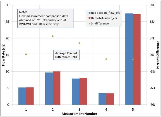
Figure 8. RemoteTracker and Mid-Section method Comparisons
