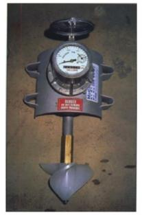
Above, propeller flow meter, the most common flow meter used for irrigation pumping plants. *Below*, flow meter installed in test section used for this study.
