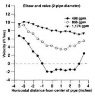
Fig. 4. Water velocity profiles under an elbow and a partially closed butterfly valve.
